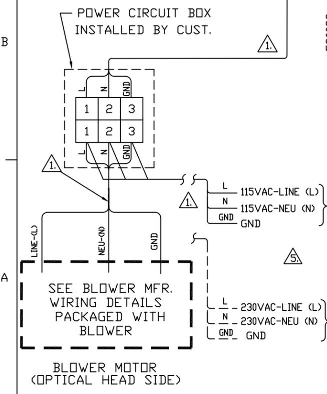
AC SERVICE ENTRANCE CIRCUIT #1 (TO BE SUPPLIED BY CUSTOMER) 1 POLE, 5 AMP CIRCUIT BREAKER WITH HI INDUCTIVE INRUSH CURRENT DELAY (42 CFM BLOWER)
