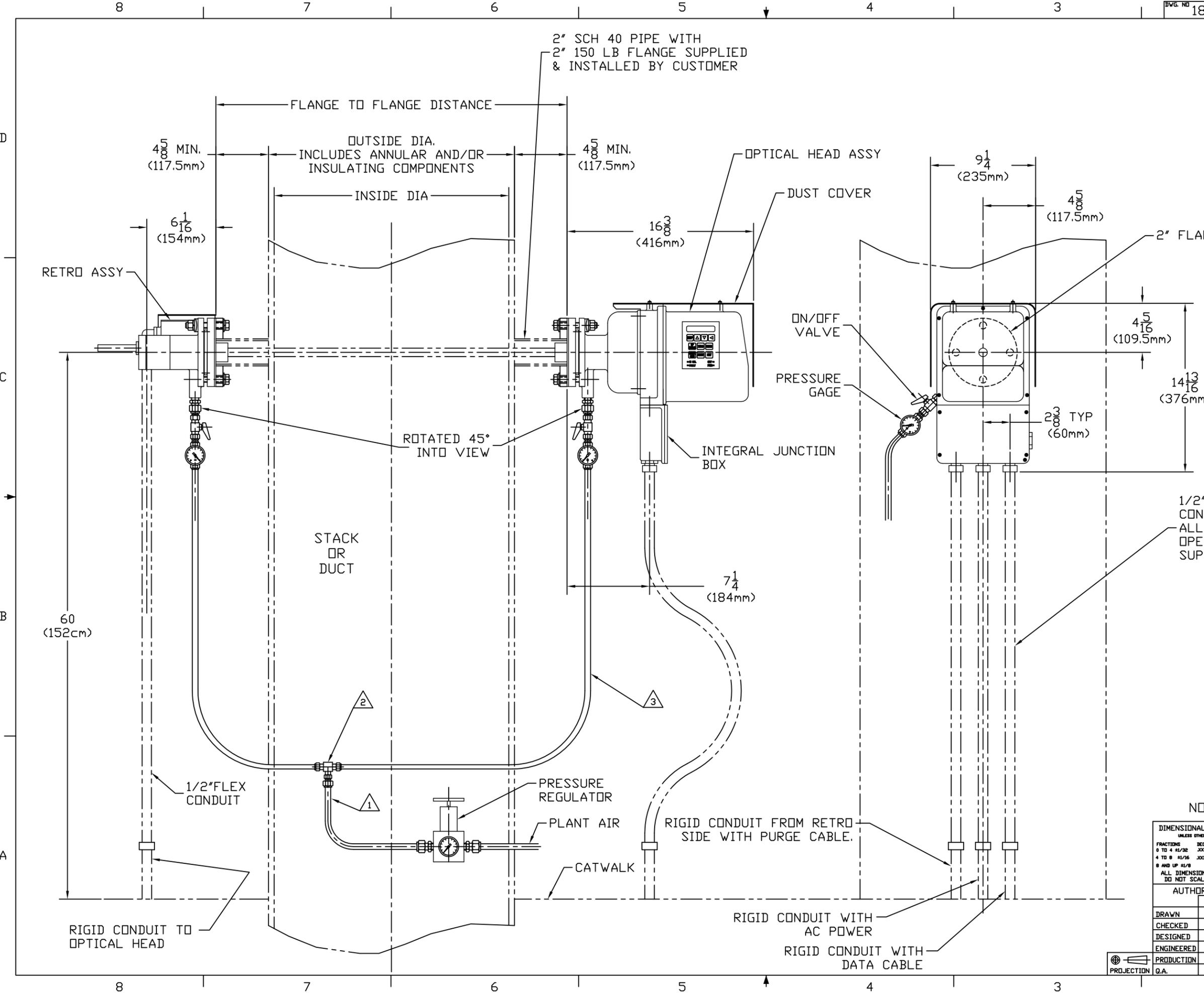
1/2" FLEX CONDUIT (TYPE EF), 3 PLACES. CONDUIT MUST HAVE ENOUGH SLACK TO ALLOW THE OPTICAL HEAD TO SWING OPEN TO THE RIGHT FOR SERVICING. SUPPLIED AND INSTALLED BY CUSTOMER
