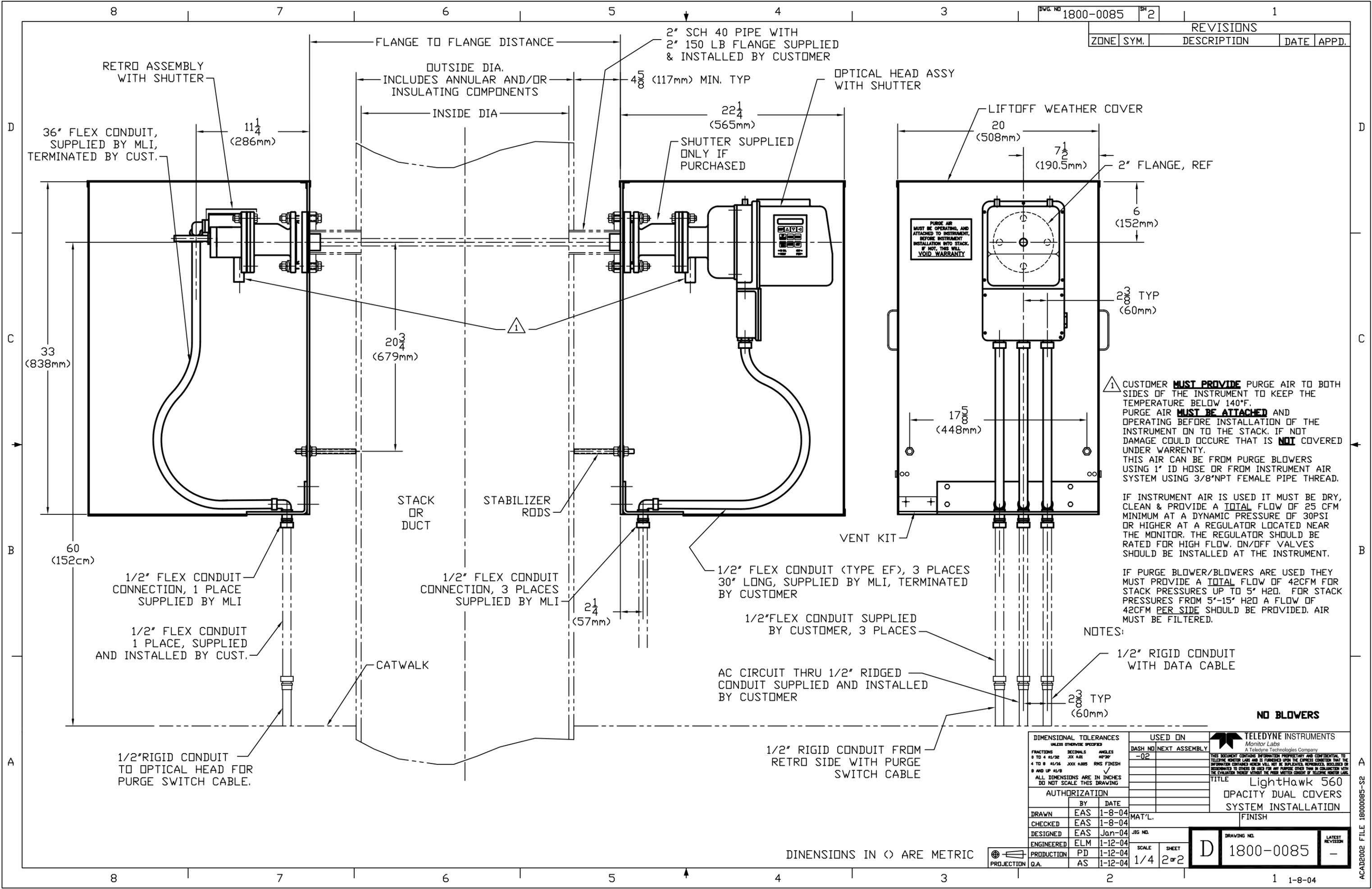
△ CUSTOMER **MUST PROVIDE** PURGE AIR TO BOTH SIDES OF THE INSTRUMENT TO KEEP THE TEMPERATURE BELOW 140°F. PURGE AIR **MUST BE ATTACHED** AND OPERATING BEFORE INSTALLATION OF THE INSTRUMENT ON TO THE STACK. IF NOT DAMAGE COULD OCCURE THAT IS **NOT** COVERED UNDER WARRENTY. THIS AIR CAN BE FROM PURGE BLOWERS USING 1" ID HOSE OR FROM INSTRUMENT AIR SYSTEM USING 3/8"NPT FEMALE PIPE THREAD.
