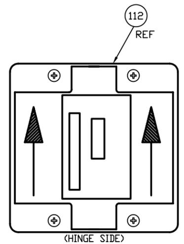
BASEPLATE FOR AI-10 MODULE WITH MODULE REMOVED
